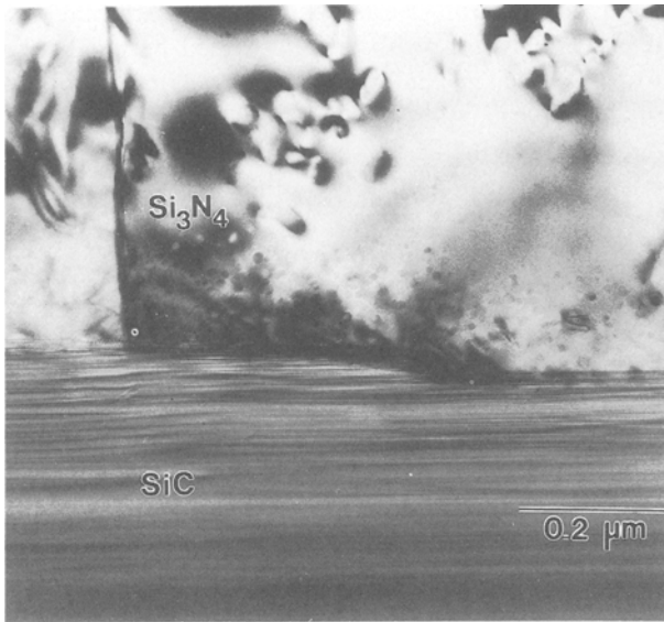
Figure 7 Bright-field transmission electron micrograph of SiC single crystal-CVD Si 3 N 4 macroscopic interface.
